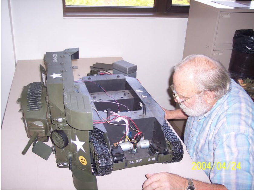
Fig. 5: Replacement of Internal RC Control Board with a WiFi-controlled Platform
